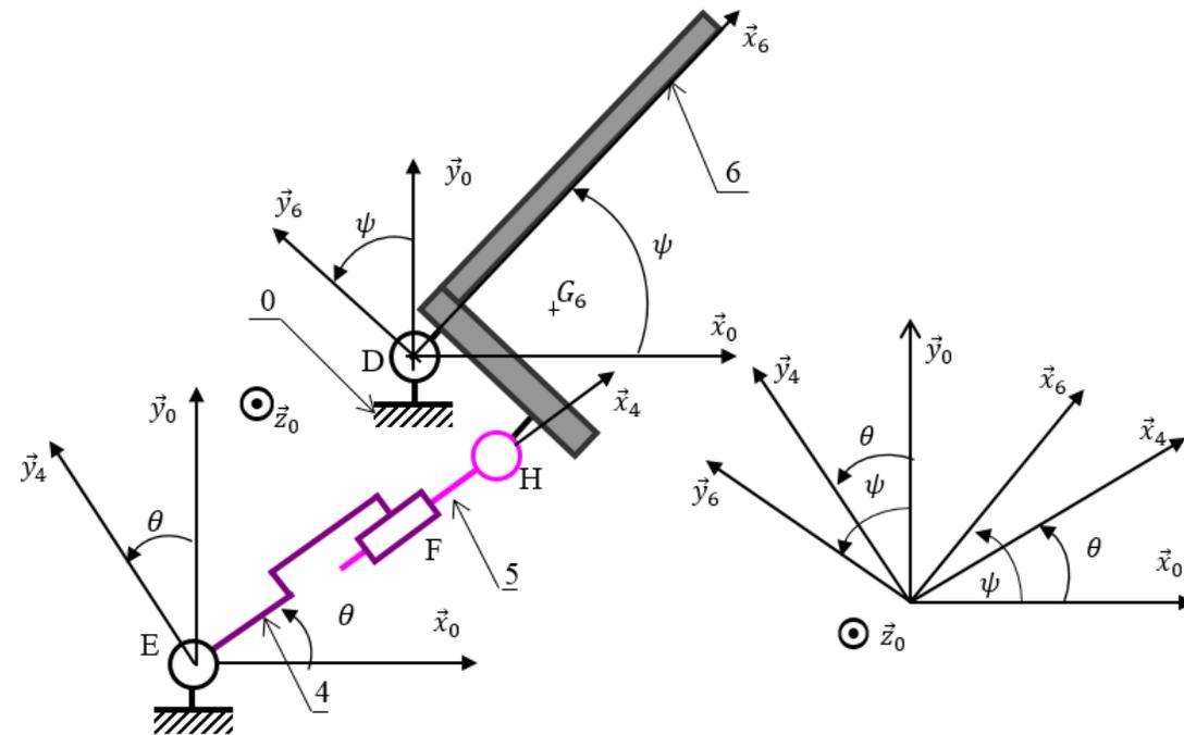
$$\begin{aligned} \overrightarrow{ED} &= e\vec{x}_0 + f\vec{y}_0, \quad \overrightarrow{HD} = h\vec{y}_6, \\ \overrightarrow{FH} &= \mu\vec{x}_4, \quad \overrightarrow{EF} = d\vec{x}_4 \end{aligned}$$
