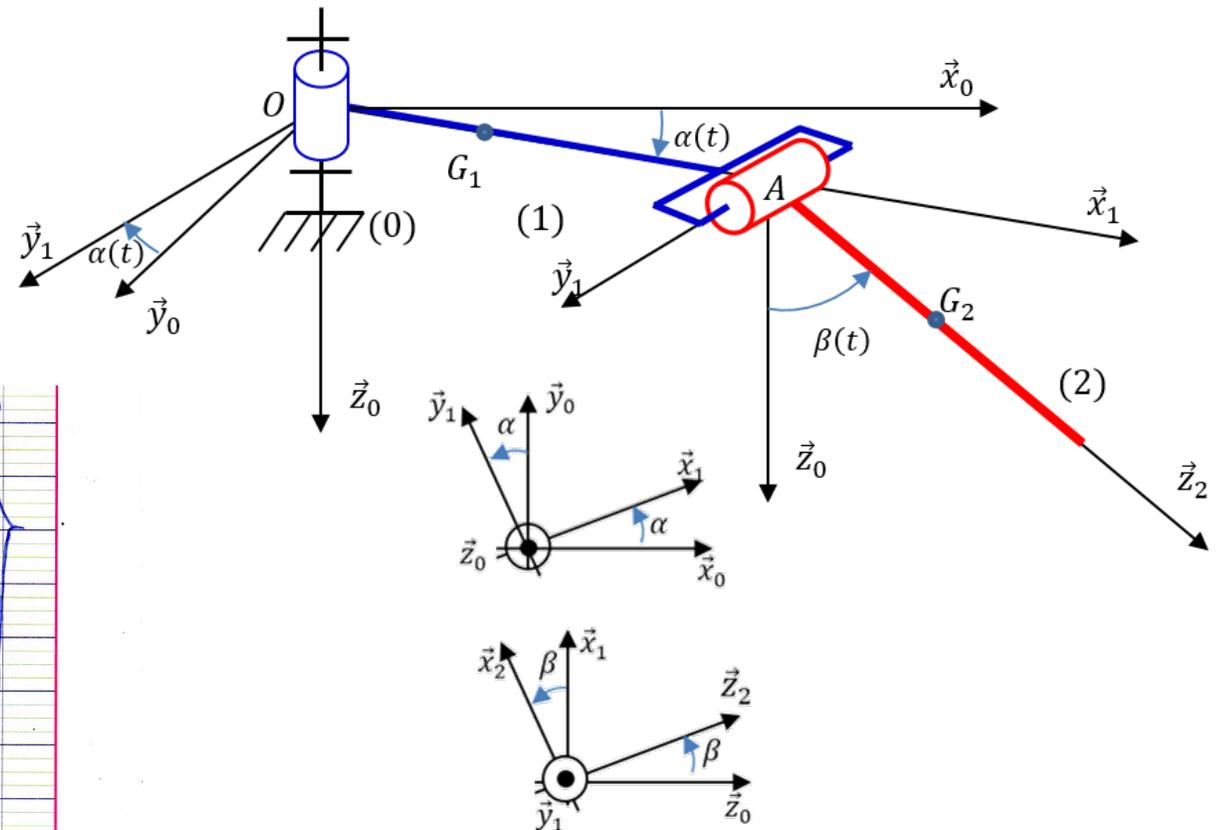
$$\{e(2|0)\}_A = \left\{ \begin{array}{l} m_2 \omega (a + b \sin \beta) \vec{y}_1 + m_2 b \dot{\beta} \vec{x}_2 \\ -(m_2 a b + A \sin \beta) \omega \vec{x}_2 + B \dot{\beta} \vec{y}_1 \\ + C \omega \cos \beta \vec{z}_2 \end{array} \right\}$$
